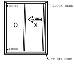
MOVE DOOR TO CLOSED POSITION AND OBSERVE WHETHER THE TOP OR BOTTOM OF PANEL CONTACTS LOCK JAMB FIRST.
